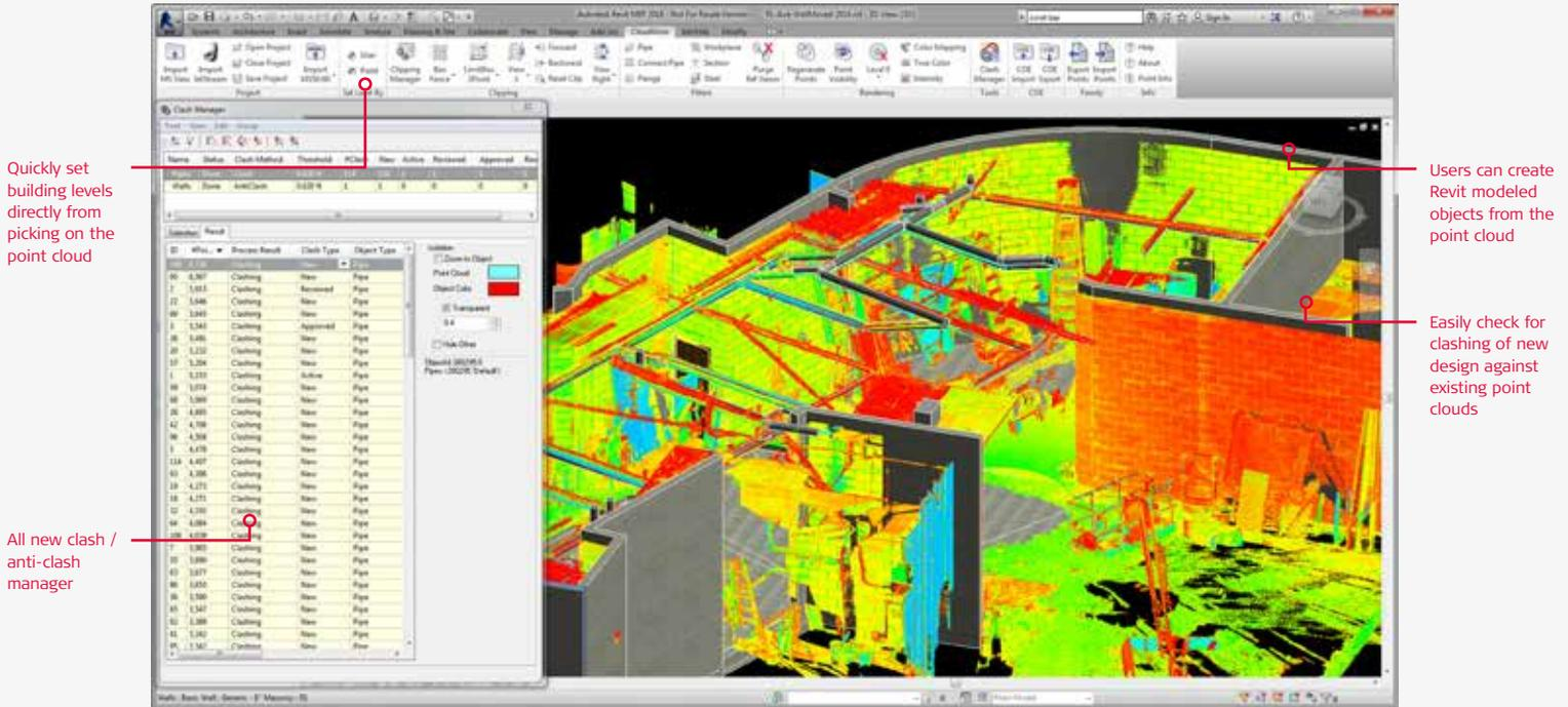
Leica CloudWorx for Revit is a breakthrough plug-in for efficiently using rich as-built point cloud data, captured by laser scanners, directly within Revit for better BIM modeling of existing buildings. This is useful for a wide range of BIM activities including retrofit design, construction and operations, and lifecycle asset management of the building. It provides a virtual visit to the site within Revit with a complete view of the captured reality.
