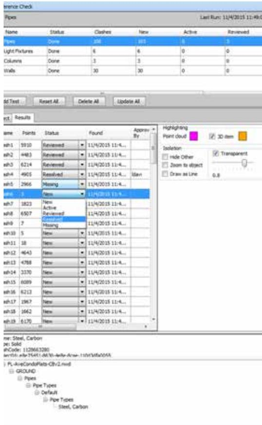
All new point cloud dash/anti-clash manager enables the user to perform interference checking against specified geometry and the point cloud.
